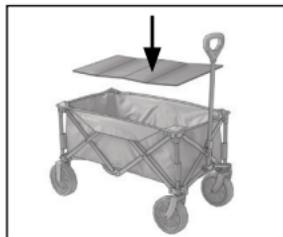
Install removable floor onto the bottom mesh panel.
